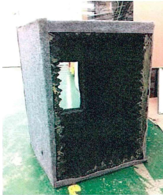
Figure 1: Acoustic Enclosure for Dill, Hand-held (Battery), Circular Steel Saw (Battery) & Grinder, Hand-Held (Battery)
